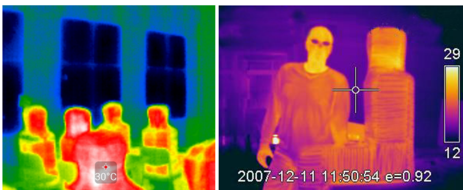
Image 4: Left: IR image of the dummies and window areas in the IATC. Right: Comparison of temperature distribution between dummy and human.
