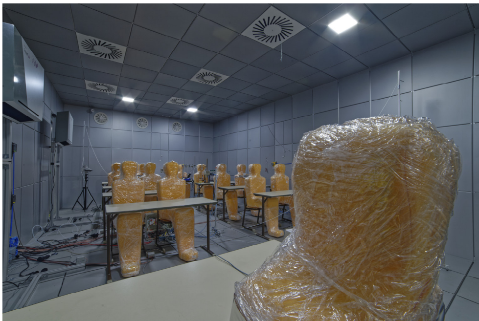
Figure 3: Structure of the SoluvaAirW air purification devices in the IATC with aerosol generator (dosing device), sensor technology and air samplers.
